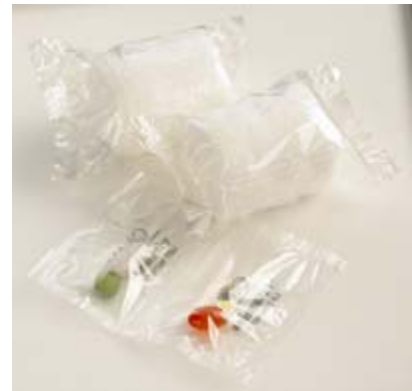
ClearFoil (aluminum-oxide coated) high barrier packages
